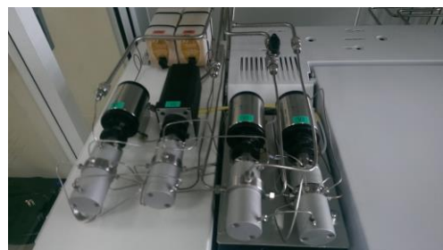
閥組件附有 purge housing 裝置極微量洩漏率( 9.9 \times 10^{-8} cc-atm/sec)
