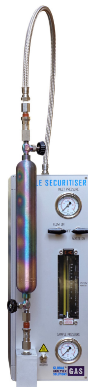
Figure 8. Sample Securitiser for liquid injection of liquified samples
