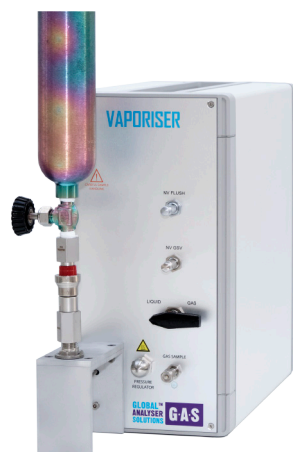
Figure 6. GAS Vaporiser for gas injection of liquified gases
